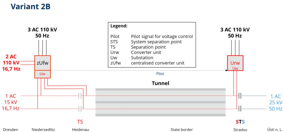
Figure 4: Variant 2B, system separation point in the Czech Republic, two-sided supply of the tunnel with AC 15 kV 16.7 Hz
