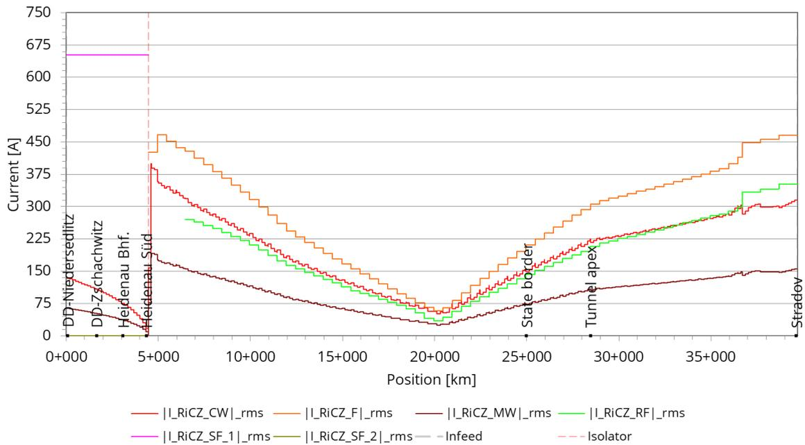
Figure 7: Maximum load currents (overhead contact line and feeder lines) in variant 2B with overhead catenary system, legend: CW – contact line, MW – messenger wire, RF – return conductor, SF – substation feeder line, F - reinforcement line (parallel to the track), RiDE – track direction to Germany, RiCZ – track direction to Czech Republic
