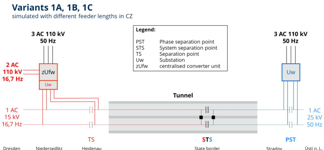
Figure 3: Variant 1, system separation point inside the tunnel apex, one-sided supply of the tunnel on both sides with AC 15 kV 16.7 Hz and AC 25 kV 50 Hz respectively
