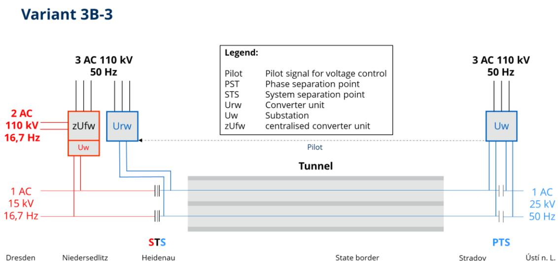
Figure 5: Variant 3B, system separation point in Germany, two-sided supply of the Erzgebirgstunnel's feeding sections with AC 25 kV 50 Hz
