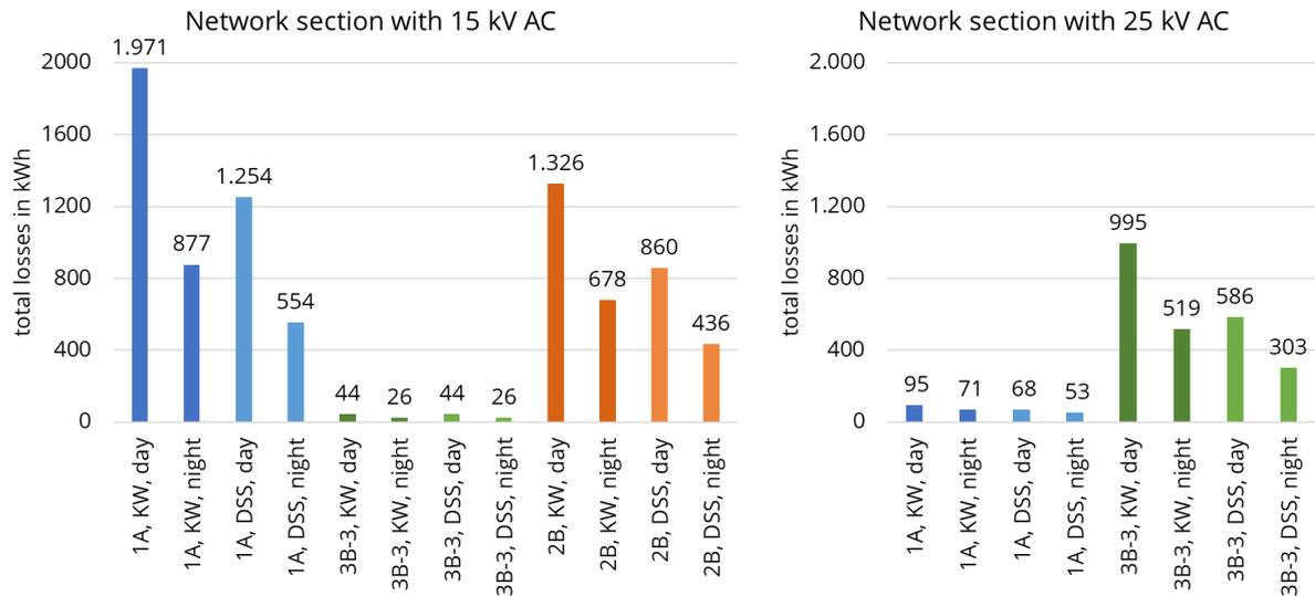
Figure 8: Total losses of the overhead contact line system (2 h simulation period, normal operation according to EBWU), legend: Variant (1A, 2B, 3B-3) according to chapter 2.1, KW – catenary system, DSS – overhead conductor rail
