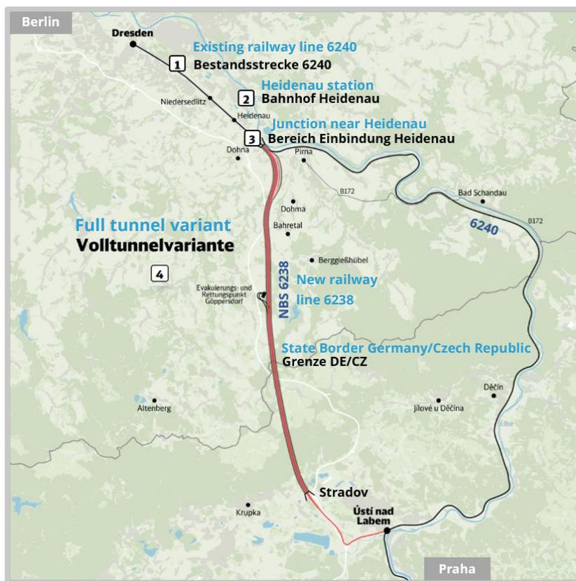
Figure 1: Route of the planned high-speed railway line Dresden – Prague (section between Dresden and Ústí nad Labem), full tunnel variant
