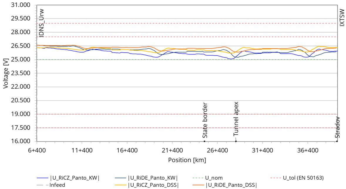
Figure 6: Comparison of voltage stability of catenary vs. overhead conductor rail, variant 3B-3 in worst-case operation, 25 kV grid component, legend: KW – catenary system, DSS – overhead conductor rail, RiDE – track direction to Germany, RiCZ – track direction to Czech Republic
